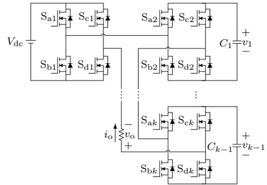
Fig. 1. Modular cascaded linear amplifier consisting of  $k$  H-bridge circuits.
