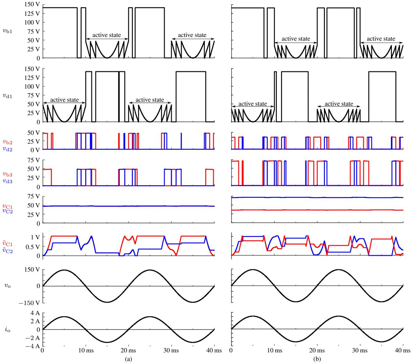
Fig. 8. Simulation waveform of the MCLA consisting of three H-bridge circuits with (a) equal and (b) unequal capacitor voltages.
