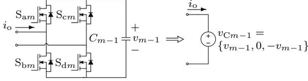
Fig. 3. Equivalent circuit of the  $m$ -th H-bridge circuit.
