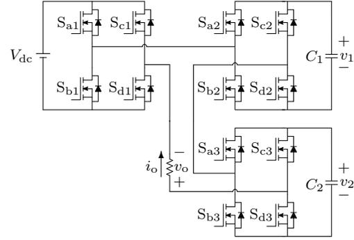
Fig. 4. Modular cascaded linear amplifier consisting of three H-bridge circuits.
