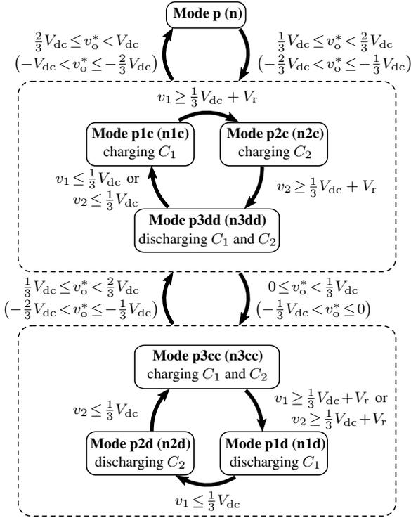
Fig. 5. Mode transition diagram for voltage balancing at  $v_{C1} = v_{C2} = V_{dc}/3$ .
