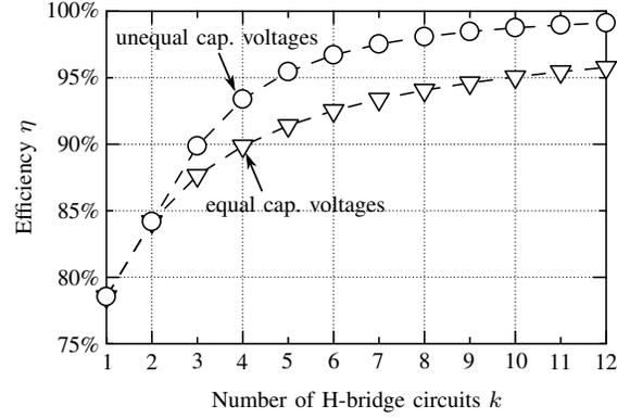
Fig. 7. Theoretical conversion efficiency of MCLA with equal and unequal capacitor voltages.
