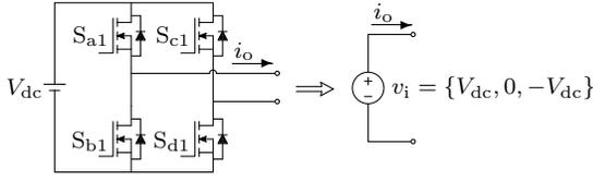
Fig. 2. Equivalent circuit of the main H-bridge circuit.
