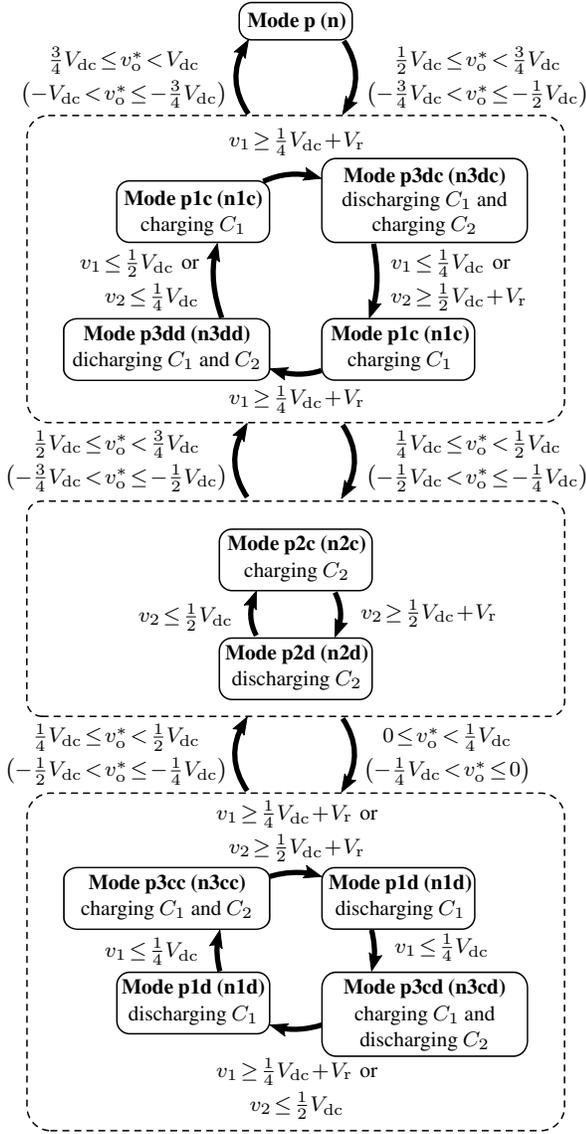
Fig. 6. Mode transition diagram of MCLA for voltage balancing at  $v_1 = V_{dc}/4$  and  $v_2 = V_{dc}/2$ .
