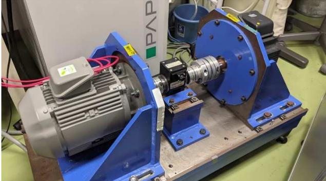
Fig. A. IM and PMM at experiment
