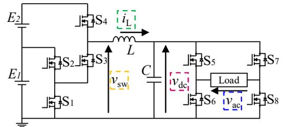
Fig. 1-a. Two battery HEECS inverter.
