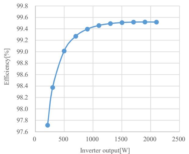
Fig. 10. Measured efficiency of proposed inverter
