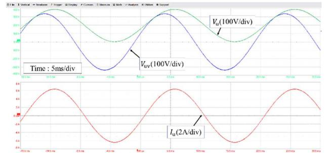
Fig. 5. Experimental waveform of  $V_u$ ,  $V_{uv}$ , and  $I_u$  ( $P_{out}=1.8 \text{ kW}$ , Resistive load)
