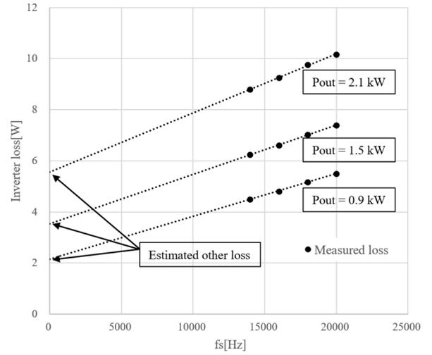
Fig. 12. Examples of how to estimate switching loss
