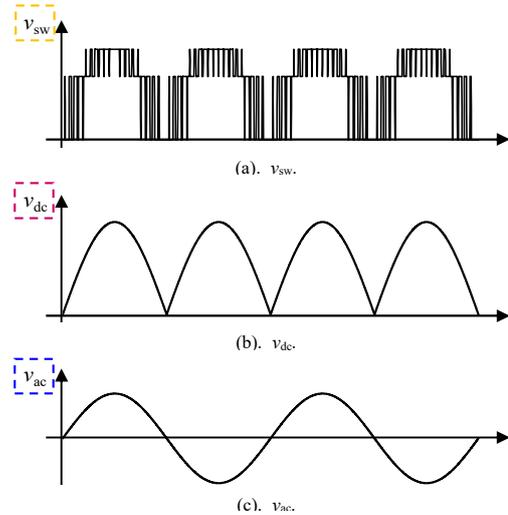
Fig. 1-b Illustration of three waveforms at circuit points in Fig. 1.
