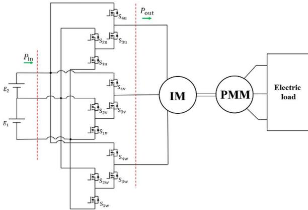
Fig. 7. IM drive with proposed inverter
