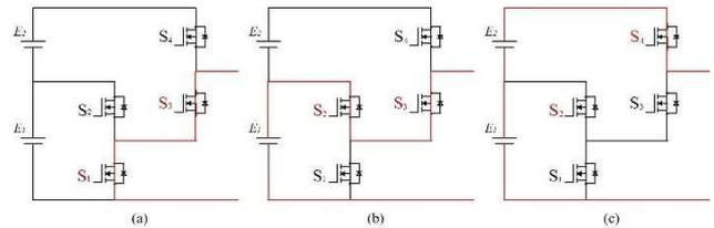
Fig. 2. Operation of 2-battery HEECS chopper
