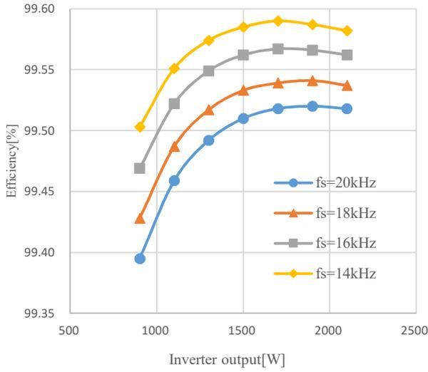
Fig. 11. Measured efficiency of proposed inverter
