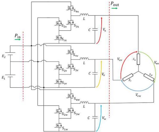
Fig. 3. Configuration of 2 battery HEECS 3-phase Inverter
