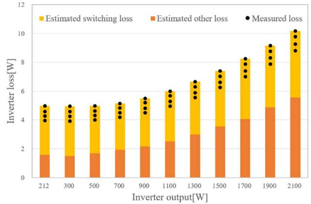
Fig. 13. Estimated loss breakdown of proposed inverter
