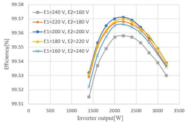
Fig. 6. Measured efficiency of proposed inverter (Resistive load, direct method<sup>[3]</sup>)
