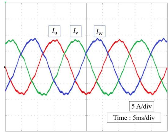
Fig. 9. Experimental waveform of current
