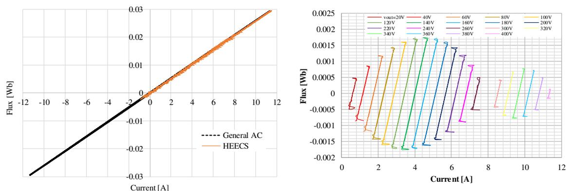
Fig. 6: Flux - current trajectory of inductor used in 2 type inverter at fundamental frequency. Fig. 7: Flux - current trajectory of inductor used in HEECS inverter at carrier frequency.
