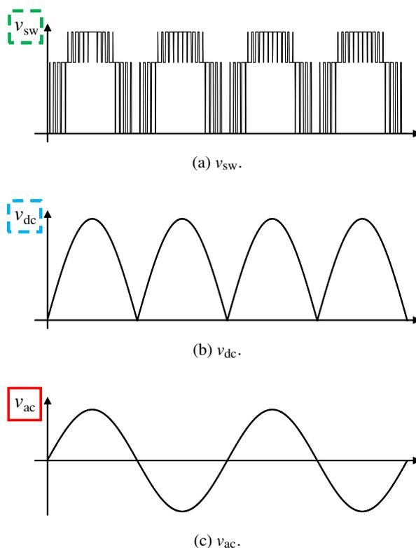
Fig. 2: Waveforms of two battery HEECS inverter.
