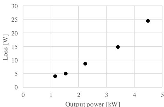
(b) Loss measurement of AC output HEECS inverter.
