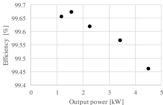
(a) AC output measured efficiency of HEECS inverter.
