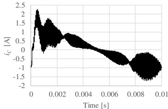
Fig. 8: Capacitor current in an half-sinusoidal operation. ( $E_1 = 279.6$  V,  $E_2 = 124.4$  V,  $R = 33.3$   $\Omega$ ,  $L = 2.43$  mH,  $C = 8$   $\mu$ F, 400 V<sub>peak</sub> AC output voltage)
