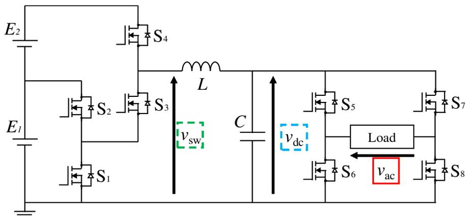
Fig. 1: Circuit of two battery HEECS inverter.
