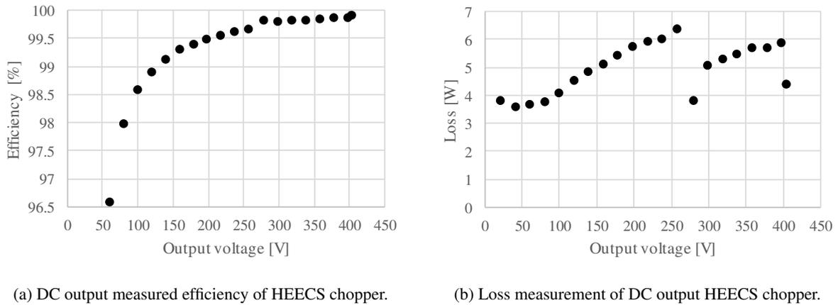
Fig. 5: Measured result of 2 HEECS inverter. ( $E_1 = 279.6$  V,  $E_2 = 124.4$  V,  $R = 33.3$   $\Omega$ ), DC output voltage)
